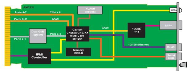
FIGURE 1. AMC221 Functional Block Diagram
